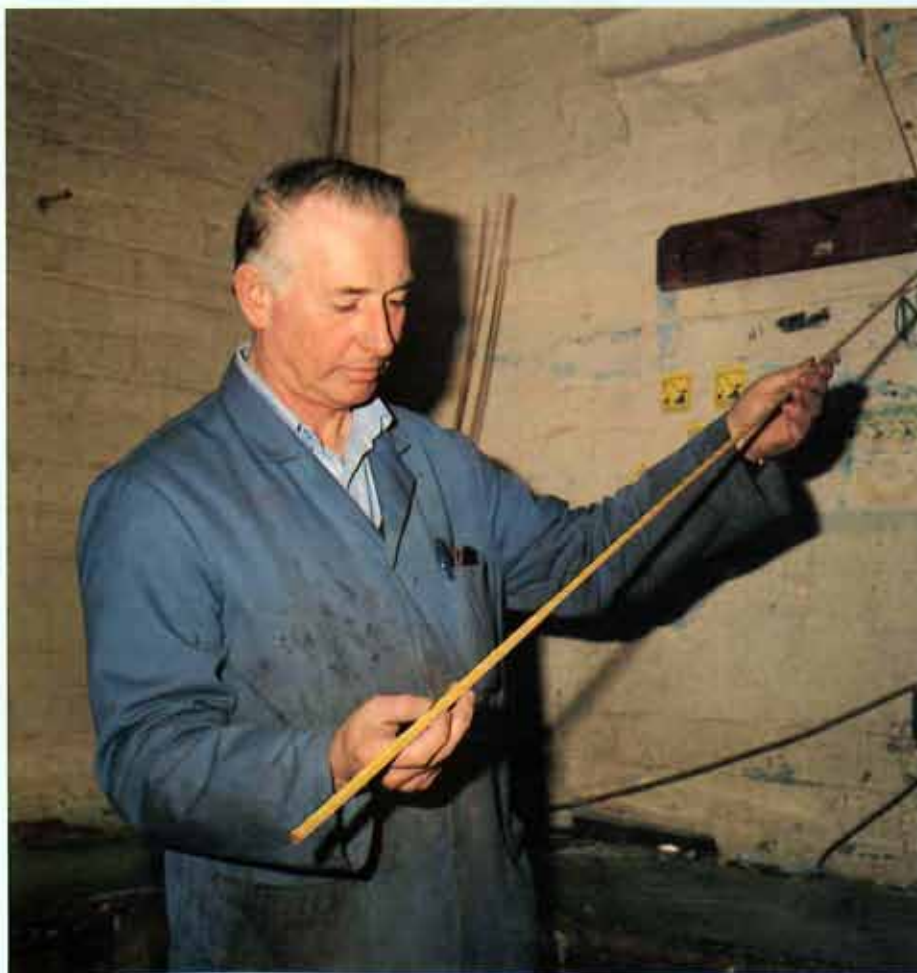
Colin Young displays a rod section glued and bound and ready for the oven.
